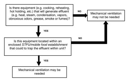
You will need to work with your regulatory authority in deciding if mechanical ventilation is required. If needed, the mechanical ventilation hood must be indicated on the layout plans of the unit.
